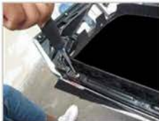
Install Step #31: Remove the grille shell metal support along bottom of grille shell.
