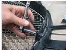
Install Step #32: Fasten GrillCraft grille to grille shell using supplied screws.
