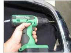
Install Step #30: Drill 3/16 inch holes for Grille mounting screws.
