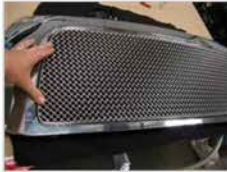
Install Step #28: Place GrillCraft grille into grille shell opening.
