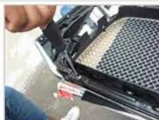
Install Step #38: Fasten support screws.
