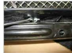
Install Step #33: Note: A clearance notch will need to be made to the metal grille support in order to clear the grille screws. Scribe the screw location onto the metal support.
