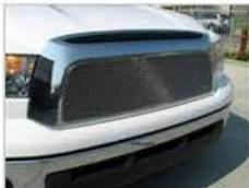
Install Step #46: 2008 Toyota Tundra shown here with GrillCraft SW Series(Woven Stainless Steel) upper mesh grille kit.
