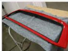
Install Step #23: The factory grille shell with center section removed.
