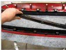
Install Step #13: Remove the grille shell metal support along the bottom of the grille shell.
