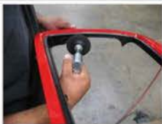
Install Step #22: Use a grinder to clean up the cut area as shown.
