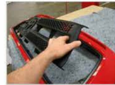
Install Step #21: Removing factory grille center bars from the grille shell.
