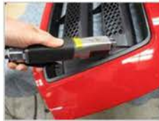
Install Step #20: Cut the factory grille center bars off.
