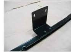
Install Step #18: The new latch bracket mounted to the grille shell support.
