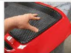
Install Step #24: Place GrillCraft grille into grille shell opening.
