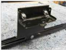
Install Step #19: Mount the original latch bracket to the new GrillCraft latch extension bracket as shown.
