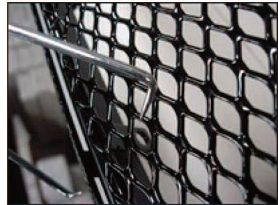
Picture #6: Place your new mesh insert into the bumper opening and mark the locations of the tabs on the grille using a sharp scribe tool. Then using a 3/16" Drill bit, drill the (5) corresponding mounting holes.
