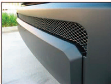
Picture #8: Place the grille back into the bumper opening and mount with the included hardware.
