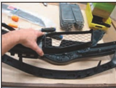
Picture #7: Removing factory grille mesh.
