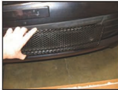
Picture #2: Place the lower grille into bumper opening from the front side.
