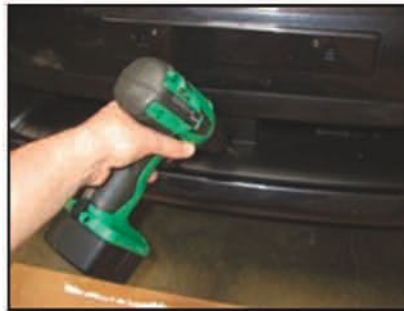
Picture #5: Drill 3/16 hole for the center mounting screw.
