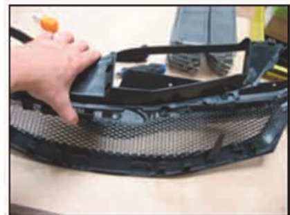
Picture #9: Reinstall the grille mesh with the grille baffles as shown.
