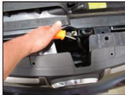
Picture #14: Fasten the grille shell screws from the back side.
