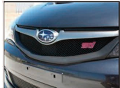
Picture #15: The StI upper MX-Series mesh grille installed.
