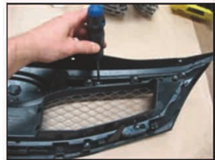
Picture #6: Remove philips screws holding the factory grille mesh.
