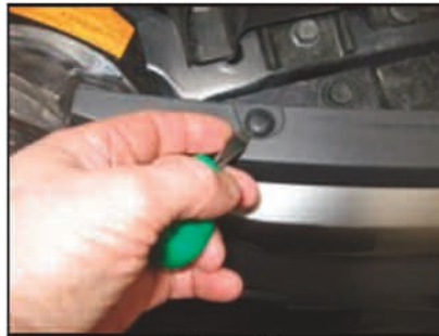
Picture #2: Start by removing the upper grille using a screw driver release the plastic grille fasteners.
