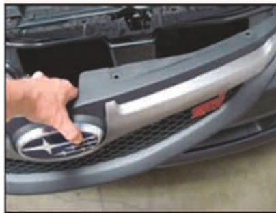
Picture #5: Remove upper grille from vehicle.
