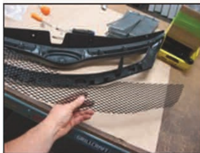
Picture #8: The center mesh replaces the factory grille mesh.
