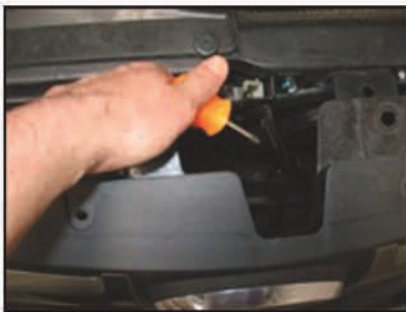
Picture #4: Remove the philips screws on the back side of the grille shell.
