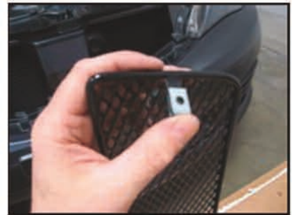
Picture #6: Attach the "U" Nuts onto the mounting tabs as shown. Now insert the grille screws from the underside but do not over tighten.
