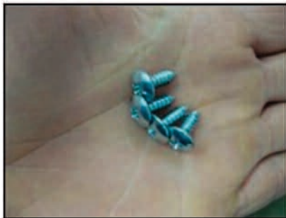
Picture #13: Use the (4) supplied philips screws when installing the upper grille shell to vehicle.
