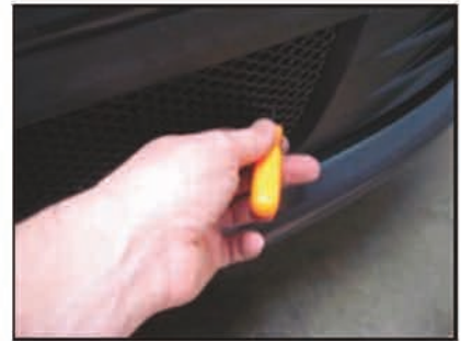
Picture #3: Using a long scribe (a long wire works great) mark mounting tab holes from the front side.
