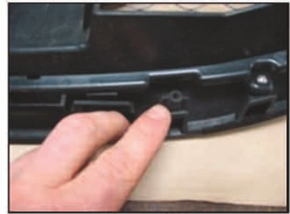
Picture #12: When reinstalling the upper grille shell use the (4) supplied philips screws.
