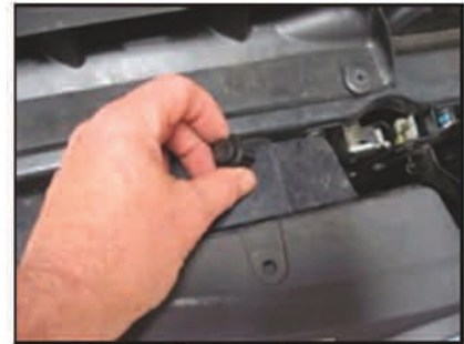
Picture #3: Start by removing the upper grille using a screw driver release the plastic grille fasteners.
