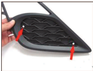
Picture #34: Note the location of the (2) holes. Repeat on other Plastic Vent Trim.
