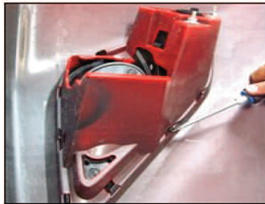
Picture #29: For Optional Side Vent Grilles, Start by removing the plastic trim for the side vents. Using a flat screw drive the tabs on the trim should pop right out.
