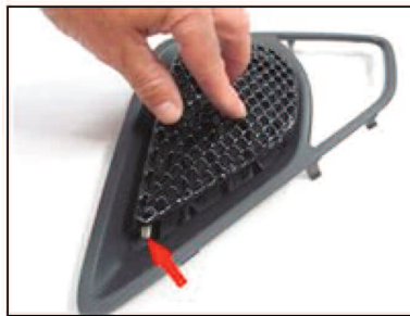
Picture #32: Align the grille into the opening and push down on the grille. This will cause the studs to make indentation in the plastic where you will need to drill (2) mounting holes.
