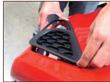
Picture #30: With all tabs unhooked, the trim should come right off of the bumper through the front.
