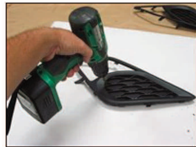
Picture #33: Using a 9/16" Drill Bit, drill (2) holes where the studs make contact with the plastic trim.
