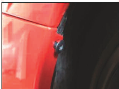
Picture #4: In the wheel-wells, you'll need to remove the upper clip holding the bumper by pushing the center of the clip inward.
