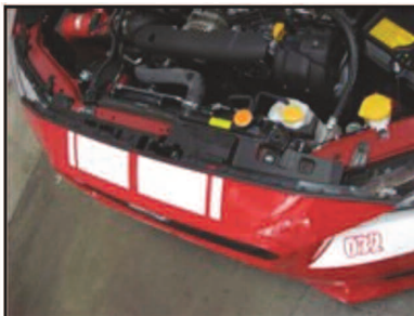
Picture #2: To perform the install you'll need to remove the bumper from the vehicle. Start by removing the 10mm bolts and Plastic Clips holding the upper part of the bumper.
