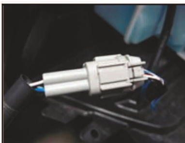
Picture #8: Disconnect the bumper-lights by pushing the center-tab inward.
