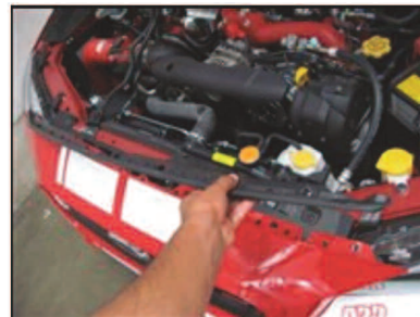
Picture #3: Once the bolts and clips are removed, the metal reinforcement bar comes right off.
