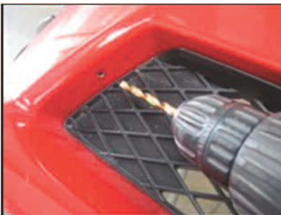
Picture #11: Use a 3/16" Drill Bit to drill the holes at the mounting locations.
