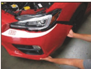
Picture #7: Once all hardware is removed, you can unclip the bumper from the vehicle by pulling towards you from the wheel-well as well as underneath the bumper.
