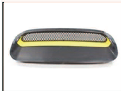
Picture #6: With the Hood Scoop removed from the vehicle, place the mesh insert through the front.
