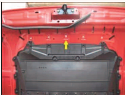
Picture #5: Once all hardware is removed, pinch the center clip in the image to lift the hood scoop away from the hood.
