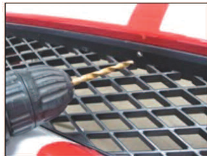
Picture #12: Use a 3/16" Drill Bit to drill the holes at the mounting locations.
