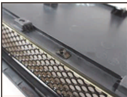
Picture #14: Install a flat-nut on the opposite end of the screw.
