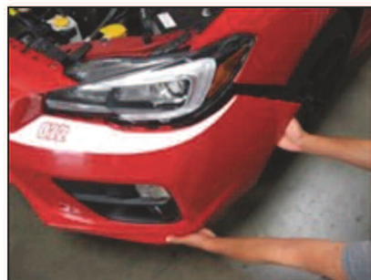
Picture #6: Once all hardware is removed, you can unclip the bumper from the vehicle by pulling towards you from the wheel-well as well as underneath the bumper.
