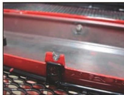
Picture #18: The top tab is notched when drilled; this is to secure the mesh to the bumper without risk of tearing the plastic tab.
