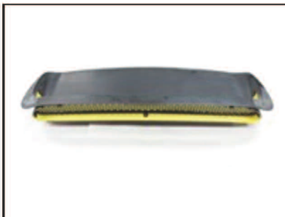
Picture #8: The side tabs sit flush with the edge of the hood scoop, and the center sits about a 3/16" away from the edge.
