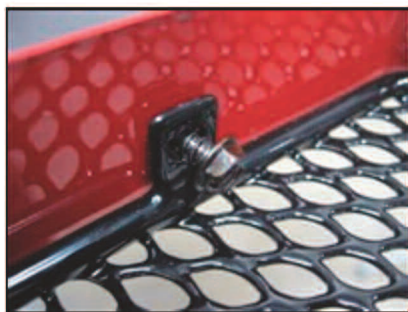
Picture #16: With the mesh insert back in place, use the included hardware to mount the insert in place.
