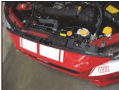
Picture #2: To perform the install you'll need to remove the bumper from the vehicle. Start by removing the 10mm bolts and Plastic Clips holding the upper part of the bumper.
