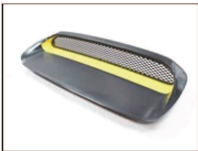
Picture #11: Re-install the mesh insert back into the hood scoop.
