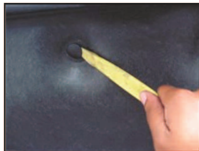
Picture #3: Use a plastic pry-tool or flat blade screw driver to remove the clips.
