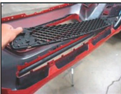
Picture #14: Once all tabs are released, the insert comes right off.
