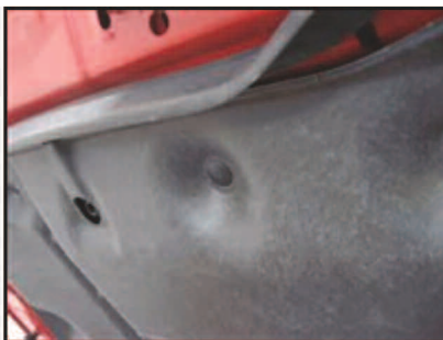
Picture #2: Under the hood, you'll need to partially-remove the sound dampener by removing the upper clips holding it in place.
