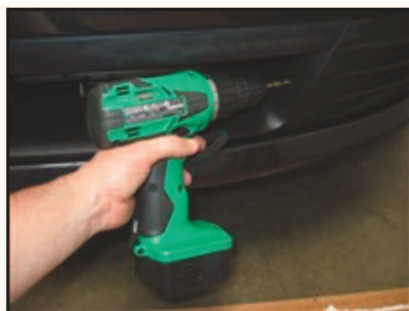
Picture #4: Drill 3/16 hole for the right & left mounting screws.
