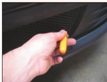
Picture #3: Using a long scribe (a long wire works great) mark mounting tab holes from the front side.
