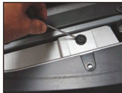
Picture #3: Remove the plastic fastners securing the top of the bumper cover as well.
