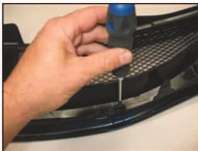
Picture #5: Fasten grille mesh screws.
