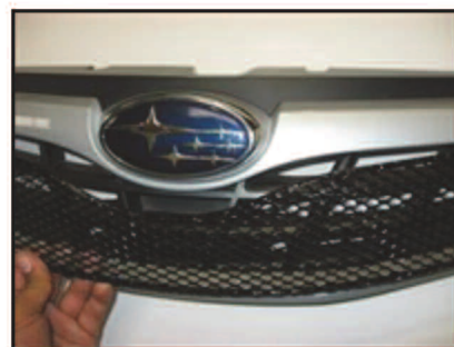
Picture #9: Place insert into grille opening. OPTIONAL: The factory grille center can be cut out. When cutting out grille center do not cut out area near mounting brackets.
