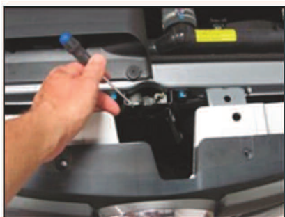
Picture #4: Remove the four screws behind the upper grille. These screws hold the upper grille to the bumper cover.
