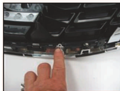
Picture #6: This is the location of the screws that we removed from the backside of the upper grille.
