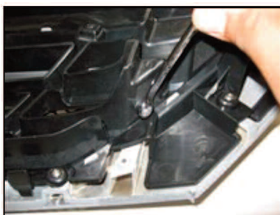
Picture #17: Fasten the grille screws.
