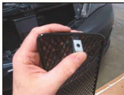
Picture #6: Attach the "U" Nuts onto the mounting tabs as shown. Now insert the grille screws from the underside but do not over tighten.
