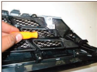
Picture #10: Using a scribe mark mounting bracket center hole location.
