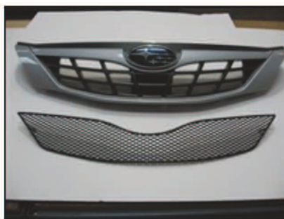
Picture #8: The insert fits into the factory grille shell. On our project vehicle we painted the upper grille surround the same color as the vehicle.
