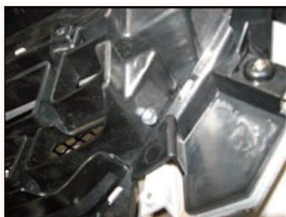
Picture #16: A view of the mounting screw installed.
