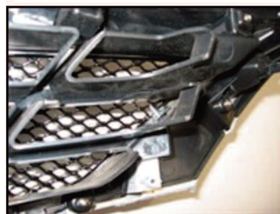
Picture #15: Mount supplied grille screws with "Flat" nuts as shown.
