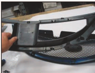
Picture #2: Remove the plastic backside baffle.
