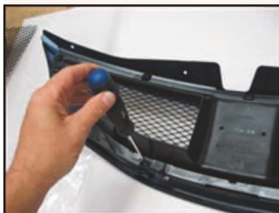
Picture #1: Remove screws from the backside of the grille.
