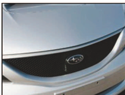
Picture #7: The factory Subaru grille with the center replacement mesh installed.
