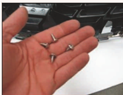
Picture #5: These are the four screws we removed from the backside of the upper grille.
