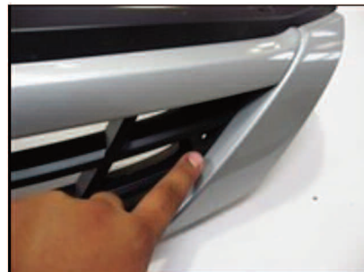
Picture #12: A look at the drilled mounting screw hole.
