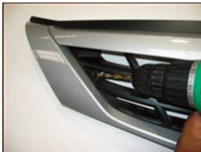
Picture #11: Drill 3/16inch holes for the mounting screws.
