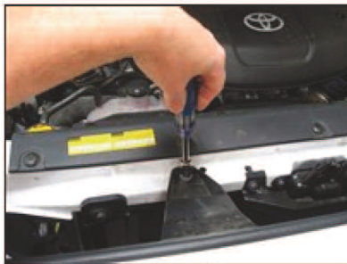
Picture #4: Remove bolts on the top of grille shell as shown.
