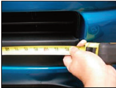
Picture #41: (OPTIONAL) Measure 18" from center drill hole. (THIS STEP FOR X-RUNNER MODEL ONLY)
