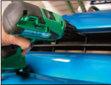
Picture #19: Drill (4) 3/16" holes for the mounting screws.
