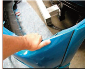
Picture #12: Remove front bumper cover. (THIS STEP FOR X-RUNNER MODEL ONLY)
