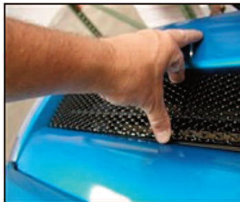
Picture #17: Press down on the grille frame as shown in photo press down in the location of mounting tabs.
