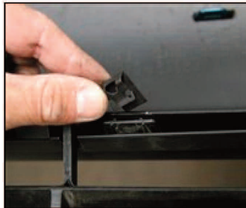
Picture #14: Remove metal "U" Clips that secure center black plastic bumper trim.(THIS STEP FOR X-RUNNER MODEL ONLY)
