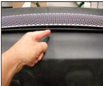
Picture #16: Place the new grille insert into bumper cover opening. Note the new grille insert is bowed.
