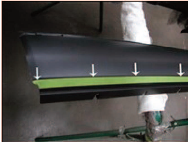
Picture #22: Another look at the trim ready to be cut note arrows this will be the cut line.(THIS STEP FOR X-RUNNER MODEL ONLY)
