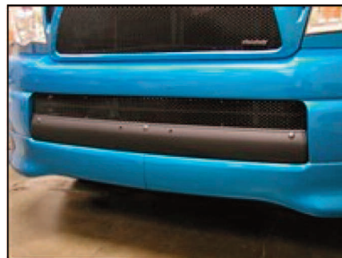
Picture #43: Tacoma X-Runner with custom upper and lower grille installed. Pictured here using (OPTIONAL) hardware kit to install black plastic center trim onto bumper.
