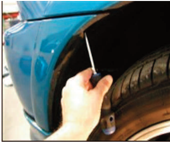
Picture #10: Remove (2) bolts located in fender well location (1) on each side..(THIS STEP FOR X-RUNNER MODEL ONLY)
