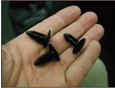
Picture #38: (OPTIONAL) Here are the clips that will hold the trim to the bumper. (THIS STEP FOR X-RUNNER MODEL ONLY)
