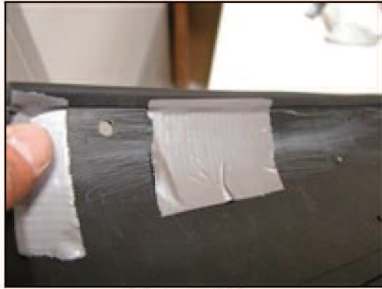
Picture #37: (OPTIONAL) Place a few strips of duct tape on the back side in order to keep rubber trim in place is a good idea. (THIS STEP FOR X-RUNNER MODEL ONLY)
