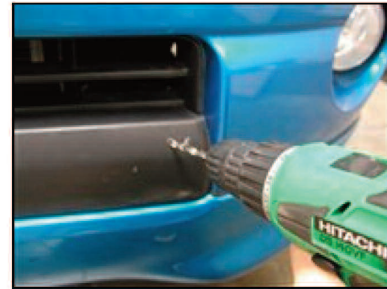
Picture #42: (OPTIONAL) Drill 1/4" hole 18" from center prong as shown. Now install supplied push clips this will hold center plastic trim onto the front bumper. (THIS STEP FOR X-RUNNER MODEL ONLY)
