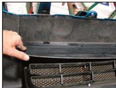
Picture #26: Place the cut trim piece in from the back side as shown.(THIS STEP FOR X-RUNNER MODEL ONLY)
