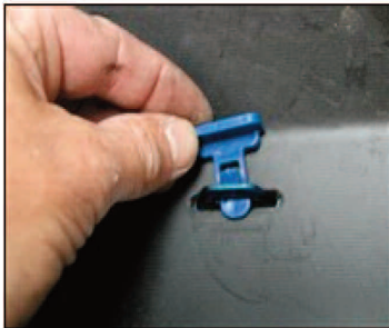
Picture #13: On the back side of the bumper cover remove blue colored clips (these hold the lower lip spoiler onto the bumper cover).(THIS STEP FOR X-RUNNER MODEL ONLY)
