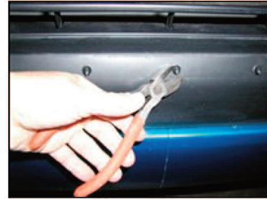
Picture #39: (OPTIONAL) Cut the center prong in the bumper using a wire cutter as shown. (THIS STEP FOR X-RUNNER MODEL ONLY)
