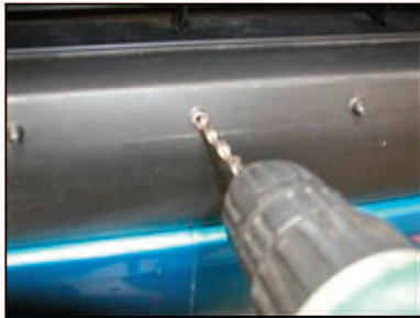
Picture #40: (OPTIONAL) Drill 1/4" hole in the center prong as shown. (THIS STEP FOR X-RUNNER MODEL ONLY)
