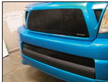
Picture #44: Tacoma X-Runner with custom upper and lower grille installed. Pictured here using (OPTIONAL) hardware kit to install black plastic center trim onto bumper.
