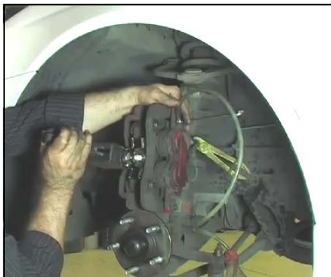
Clamp brake line before pushing pads back
