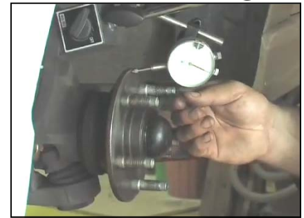
Check Hub run-out
