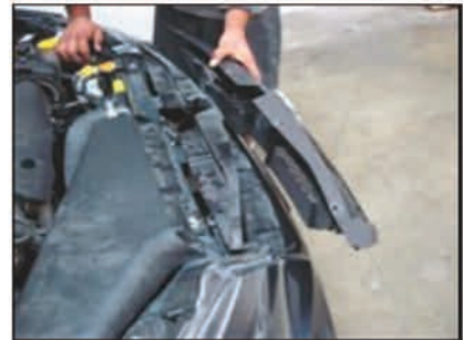
Picture #6: Once all the backside screws are removed the grille shell can then be removed from the vehicle.
