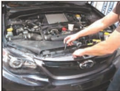
Picture #4: Pull forward on the upper grille in order to gain access to the back side of the grille shell screws.
