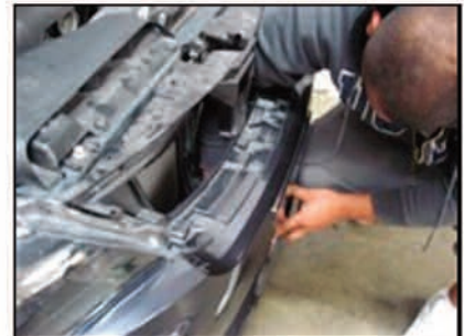
Picture #15: Gain access to the backside of the lower grille by reaching through the upper grille area and fasten screws. Next reinstall upper grille.
