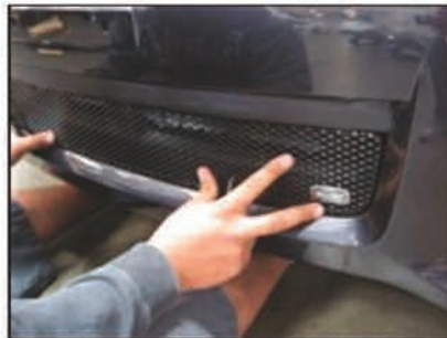
Picture #8: Hold lower grille securely in place.
