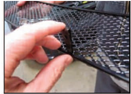
Picture #12: Attach supplied "U" nut to the center mounting tab.
