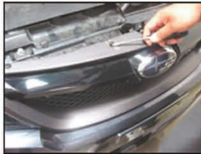
Picture #2: Remove all the plastic fasteners along the top of the grille shell.
