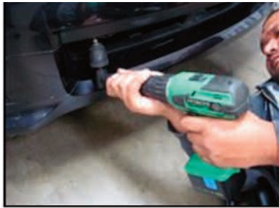
Picture #10: drill holes for mounting screws using 3/16 inch drill bit. The upper holes may require using a 90 degree drilling adapter as shown.
