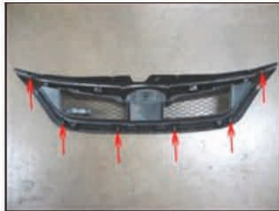
Picture #5: Shown here are the locations of the grille shell screws that must be removed.
