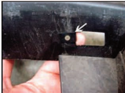
Picture #13: Attach the upper supplied "U" nuts onto the bumper plastic as shown.
