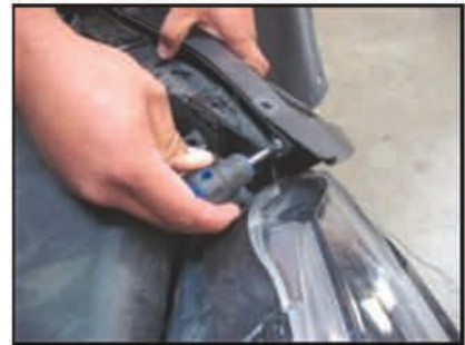
Picture #3: Remove the right & left corner screws located on the back side of the grille shell as shown using a stubby "Short" screwdriver.
