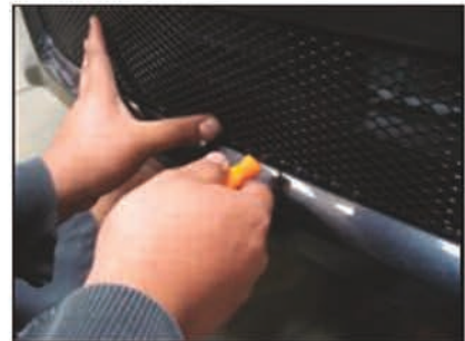
Picture #9: Using a sharp scribe mark the(3)grille mounting tab locations onto the bumper.
